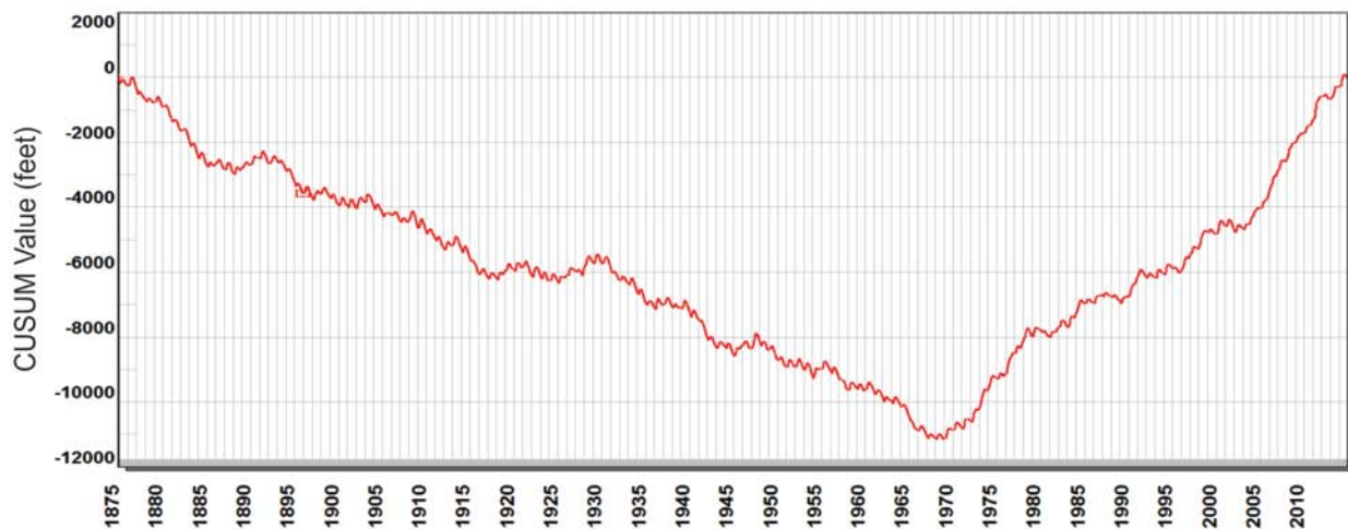
Figure 3. CUSUM Method applied to the daily mean water levels of Lake Champlain.
