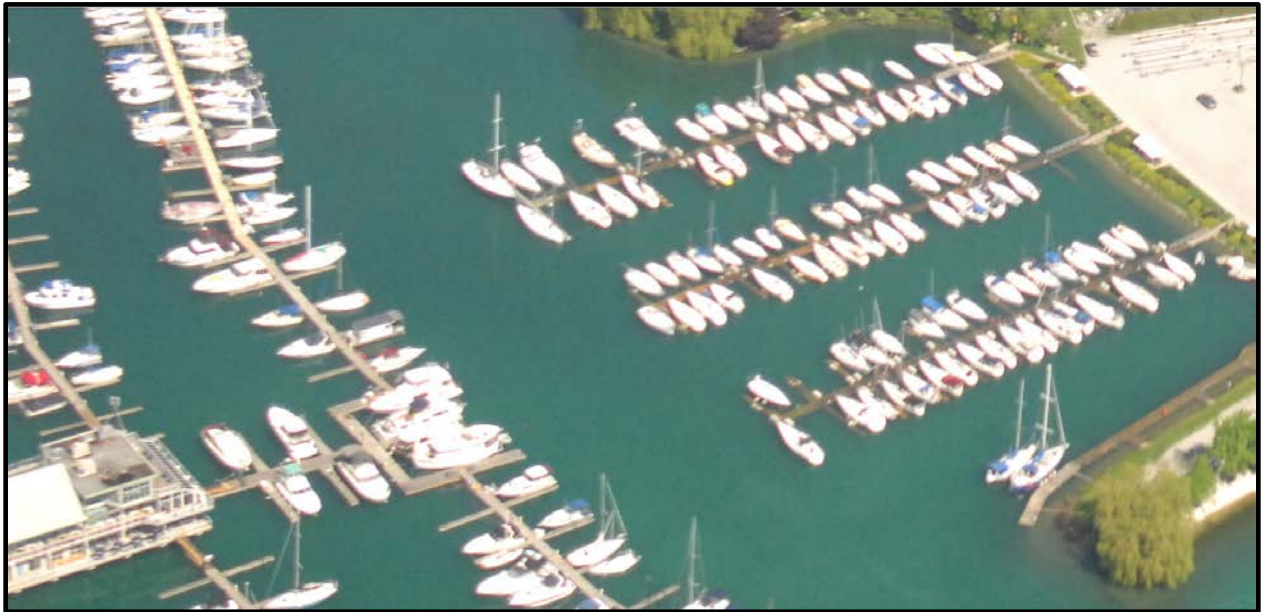
Figure 8-14: Marina facilities in Scarborough, Ontario illustrating inundation of docks (right) and docks that appear to not be inundated (left). Photo credit: Transport Canada - National Aerial Surveillance Program, June 8, 2017.
