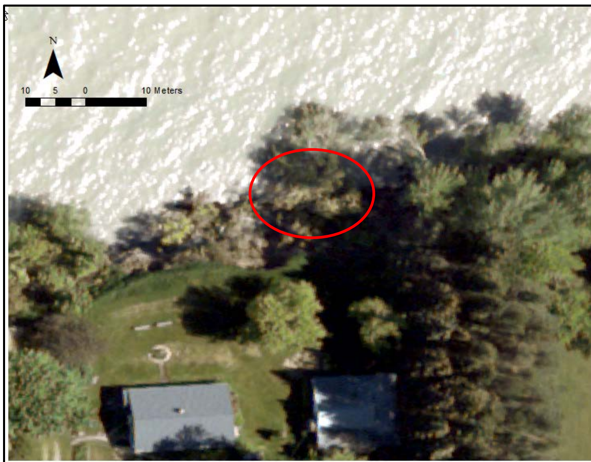
Figure 6-10: Example of shoreline erosion observed for a specific property in Niagara County. Note the trees and vegetation in the water. (Source: USACE Aerial Imagery – June 2, 2017).
