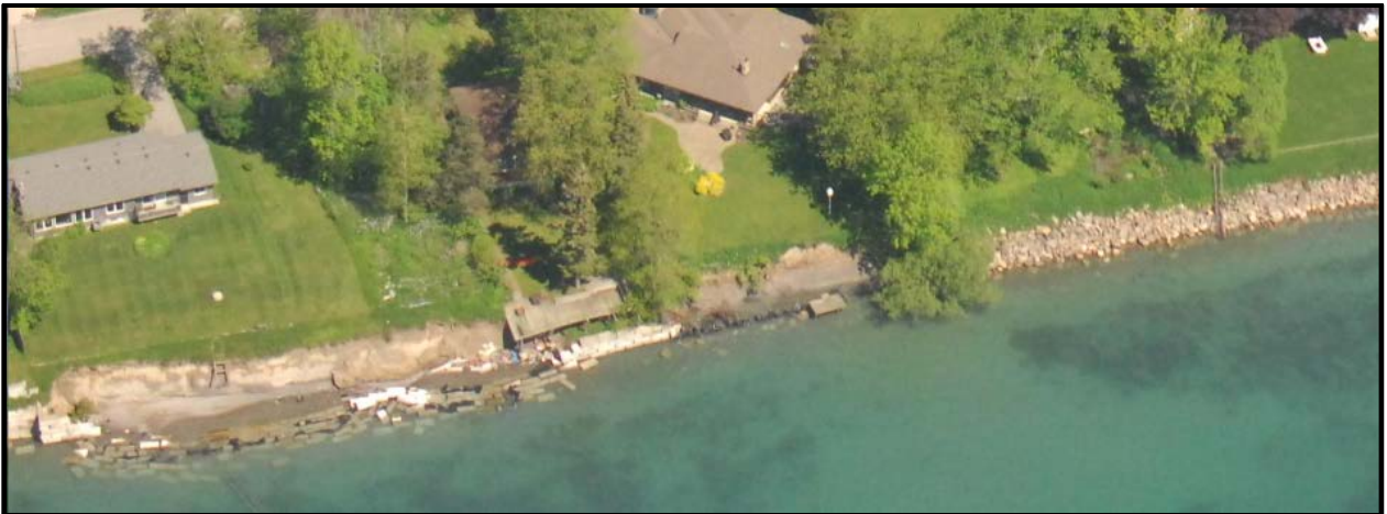
Figure 6-48: Example of collapsed shoreline protection in Ajax Ontario, June 8, 2017. Photo credit: Transport Canada National Aerial Surveillance Program.
