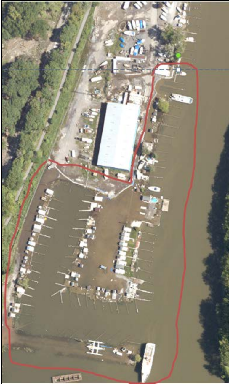
Figure 8-4: Example of inundation that can be identified through the USACE orthoimagery for Monroe County with particular issues highlighted (red = inundation of docks, nearshore area, and sandbagging) Photo credit: USACE, June 2017.
