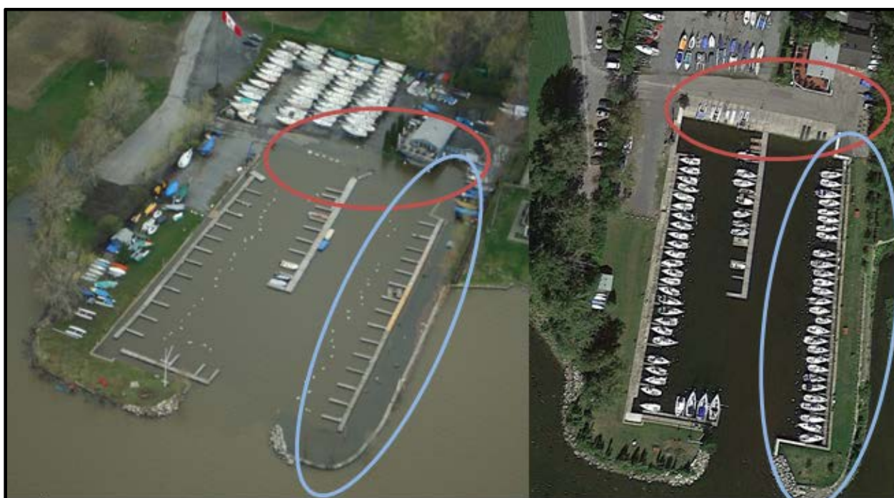
Figure 8-25: Baie-d'Urfe Yacht Club showing inundation of shoreline areas on May 8, 2017 (left) relative to lower water level conditions in September 2013 (right). Photo credit: (left) Transport Canada - National Aerial Surveillance Program, (right) Google Earth, September 17, 2013.
