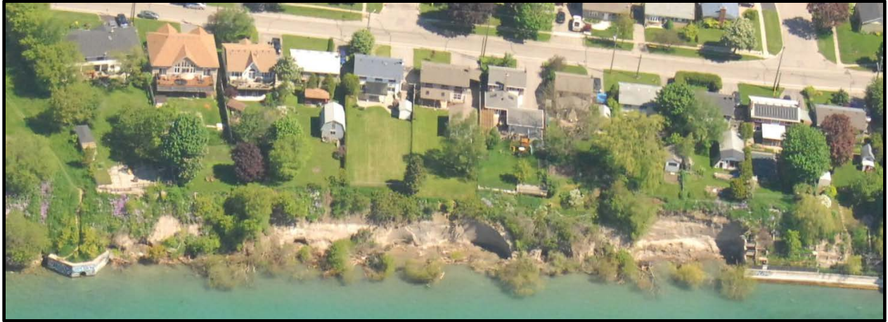
Figure 6-49: Example of shoreline erosion in Oshawa, Ontario, June 8, 2017. Photo credit: Transport Canada National Aerial Surveillance Program.
