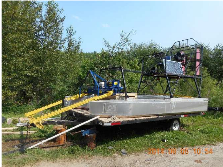
Figure 9. Airboat mounted mechanical cattail removal assembly.
