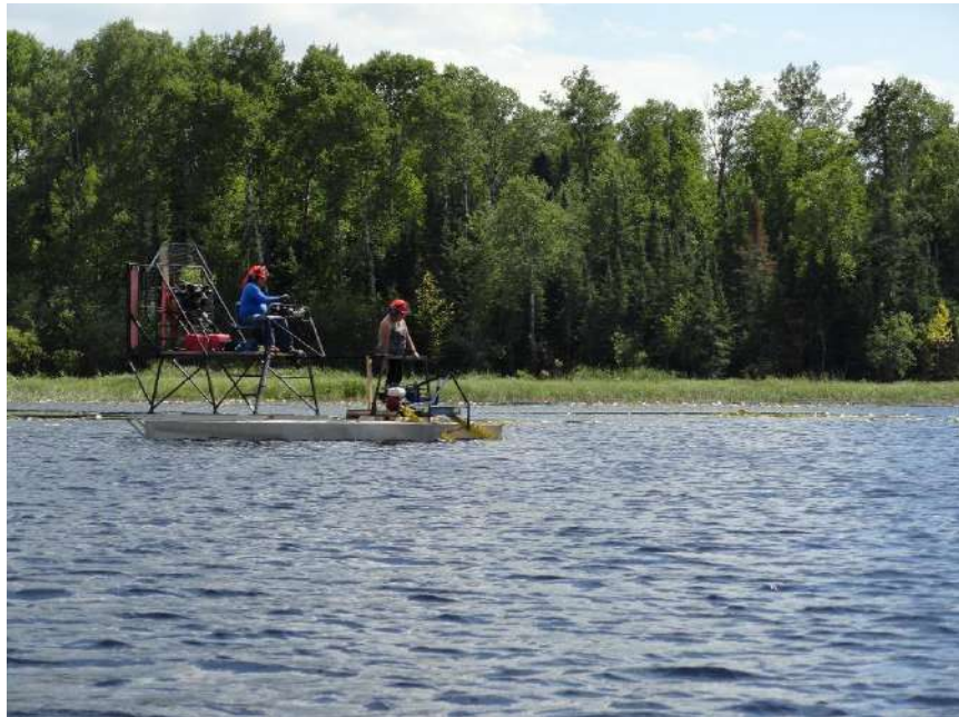
Figure 11. August 12, 2014: Using mechanical cattail removal assembly for cattail removal - after operation.
