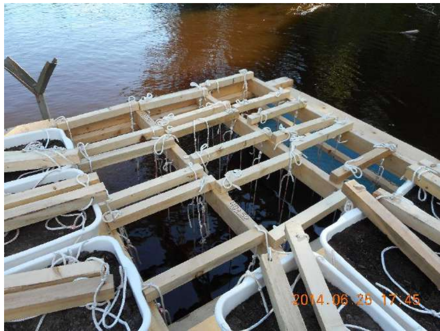
Figure 2. WR raft assembly and tubs of sediment; some deployed, some awaiting WR seedling plants.
