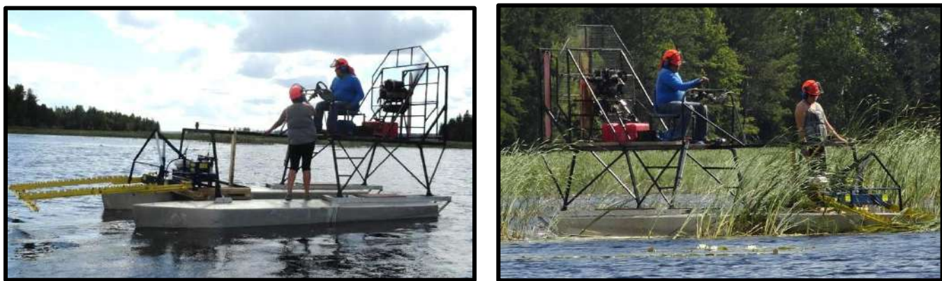
Figure 2. Cutting bar apparatus attached to the SRFN airboat (left). The bar is lowered into the water and cutting of the cattails occurs (right). The system requires both an operator for the airboat and the cutting bar.
