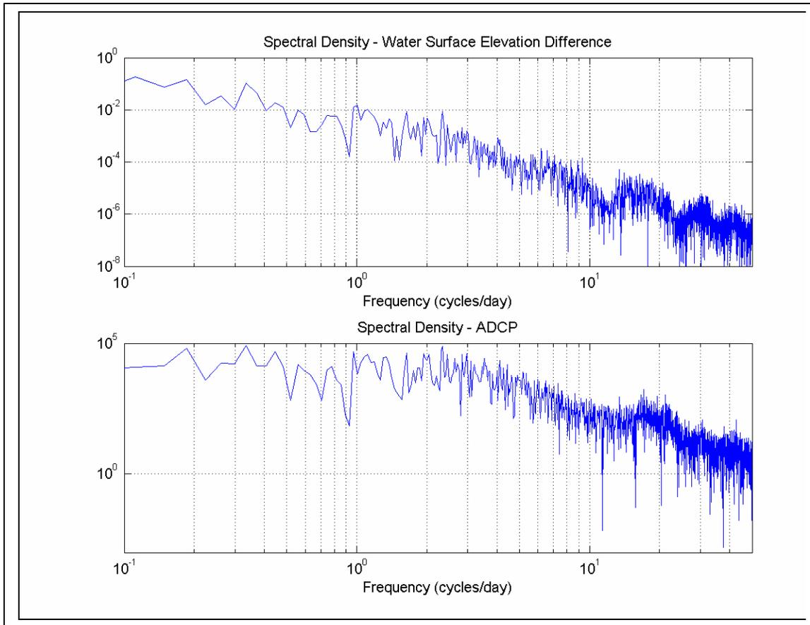
**Figure 2** Power spectral density of (a) the water surface elevation difference between the Rt. 78 causeway and the north end of Missisquoi Bay, and (b) the ADCP measured currents at the Rt. 78 causeway opening.
