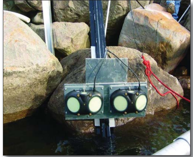
A new hydrometric (water quantity) gauging station on the St. Marys River, one of four new stations on the connecting channels of the upper Great Lakes installed under the Study. Government support for the continued operation of these stations after the Study is completed will provide key data to help Canada and the U.S. manage the Great Lakes under a changing climate regime.
