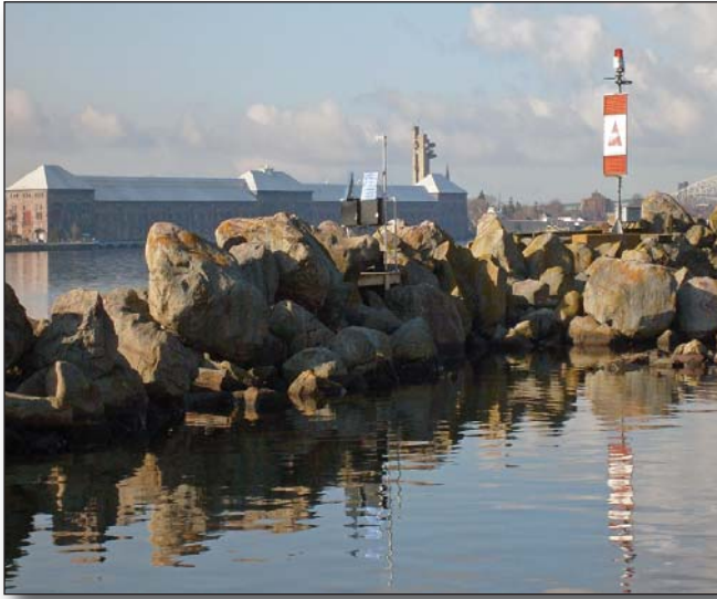
A new hydrometric (water quantity) gauging station on the St. Marys River, one of four new stations on the connecting channels of the upper Great Lakes installed under the Study. Government support for the continued operation of these stations after the Study is completed will provide key data to help Canada and the U.S. manage the Great Lakes under a changing climate regime.
