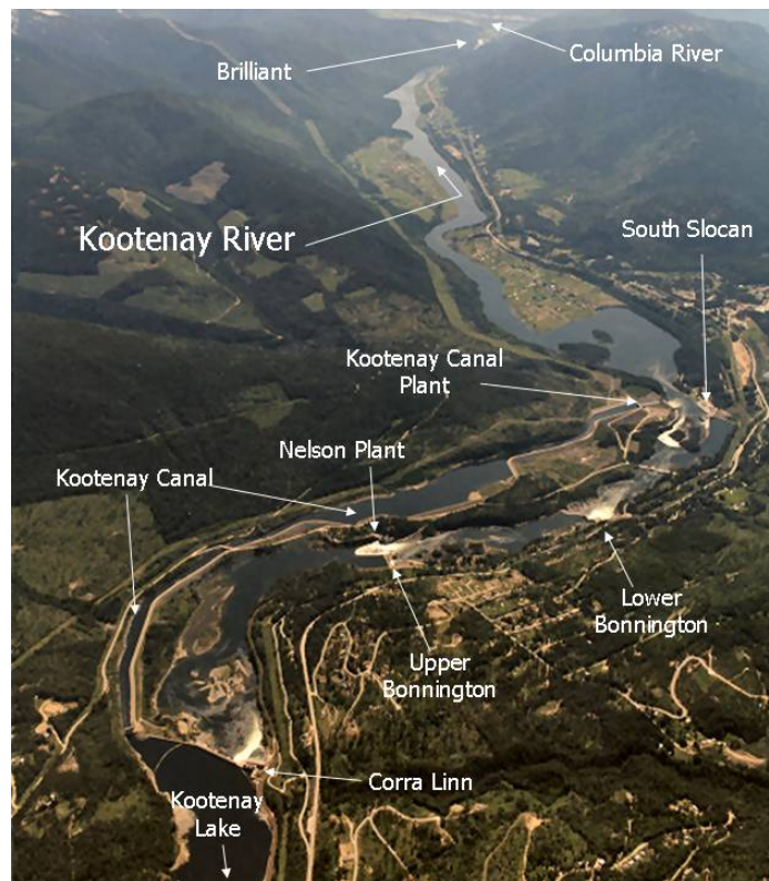
The Kootenay Canal parallels the main channel of the lower Kootenay River for four kilometres. Six hydroelectric plants mark this section of the river.
