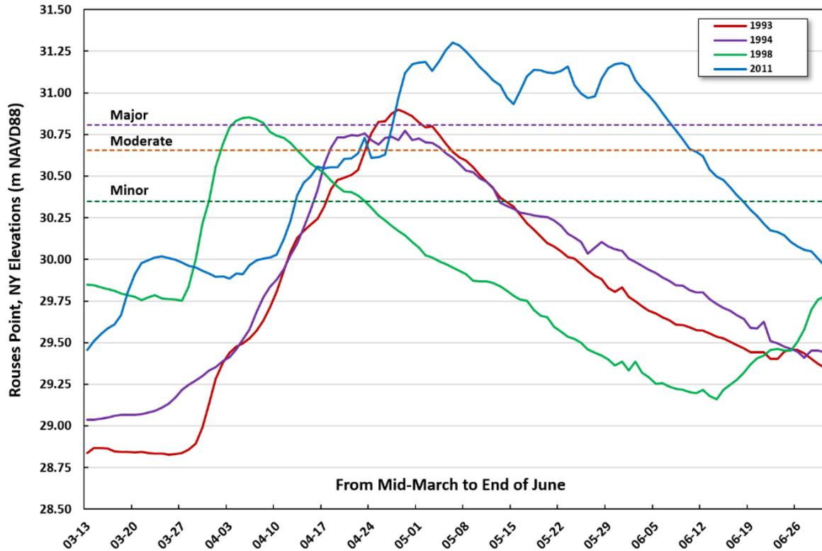
Figure 3. Spring water levels at Rouse's Point, New York during Lake Champlain major floods, 1990-2019. <sup>4</sup>
