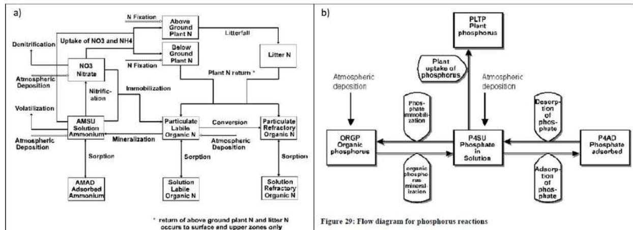
Figure 4-11. Conceptualized nitrogen (a) and phosphorus (b) processes in HSPF (Bicknell et al., 1997). *Permission for use of image will be requested prior to public release.*
