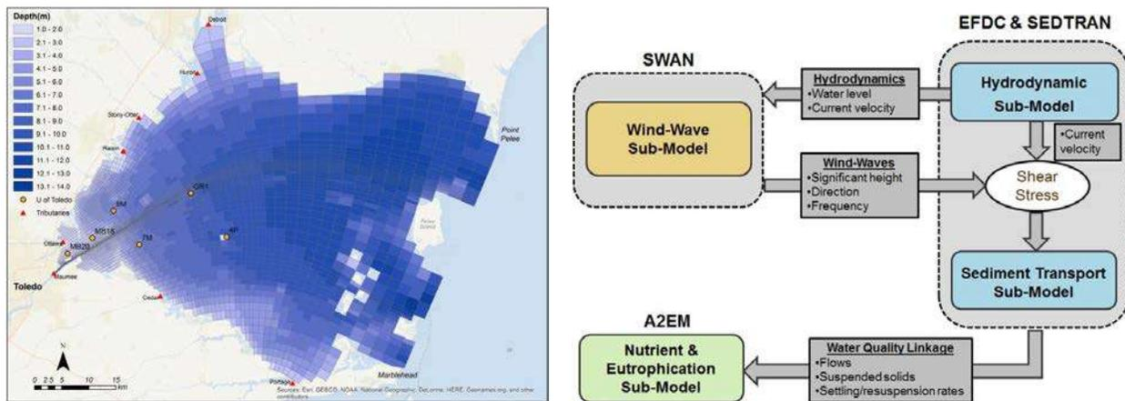
Figure 4-15. Model grid area and schematic diagram of WLEEM.
