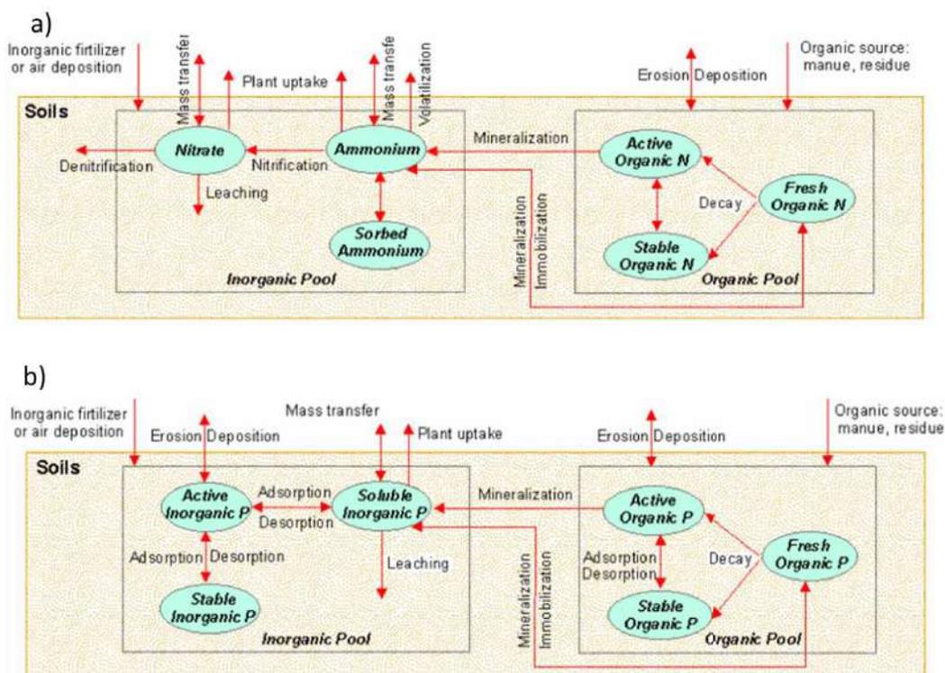
Figure 4-12. Conceptualized nitrogen (a) and phosphorus (b) soil processes in the Nutrient Sub-Module (Johnson et al., 2006). *Permission for use of image will be requested prior to public release.*
