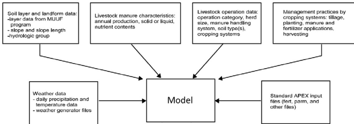
Figure 4-10. Example input structure for APEX (adapted from Gassman et al., 2010)
