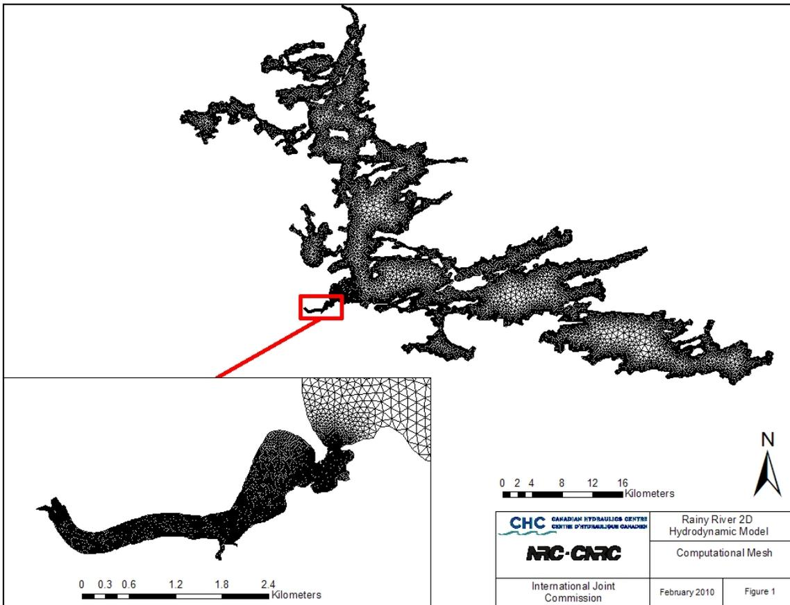
Figure B-1 - 2D Computational Mesh (Mesh 1)
