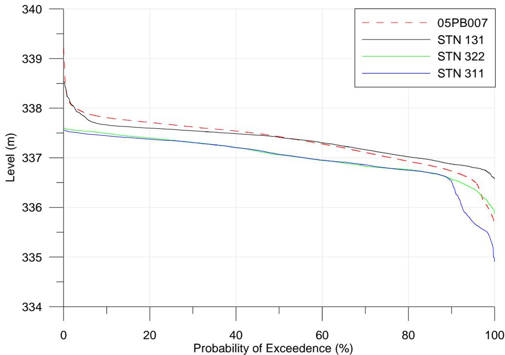
**Figure 3-4 - Elevation Duration Curves for EC Lake Level Data**
