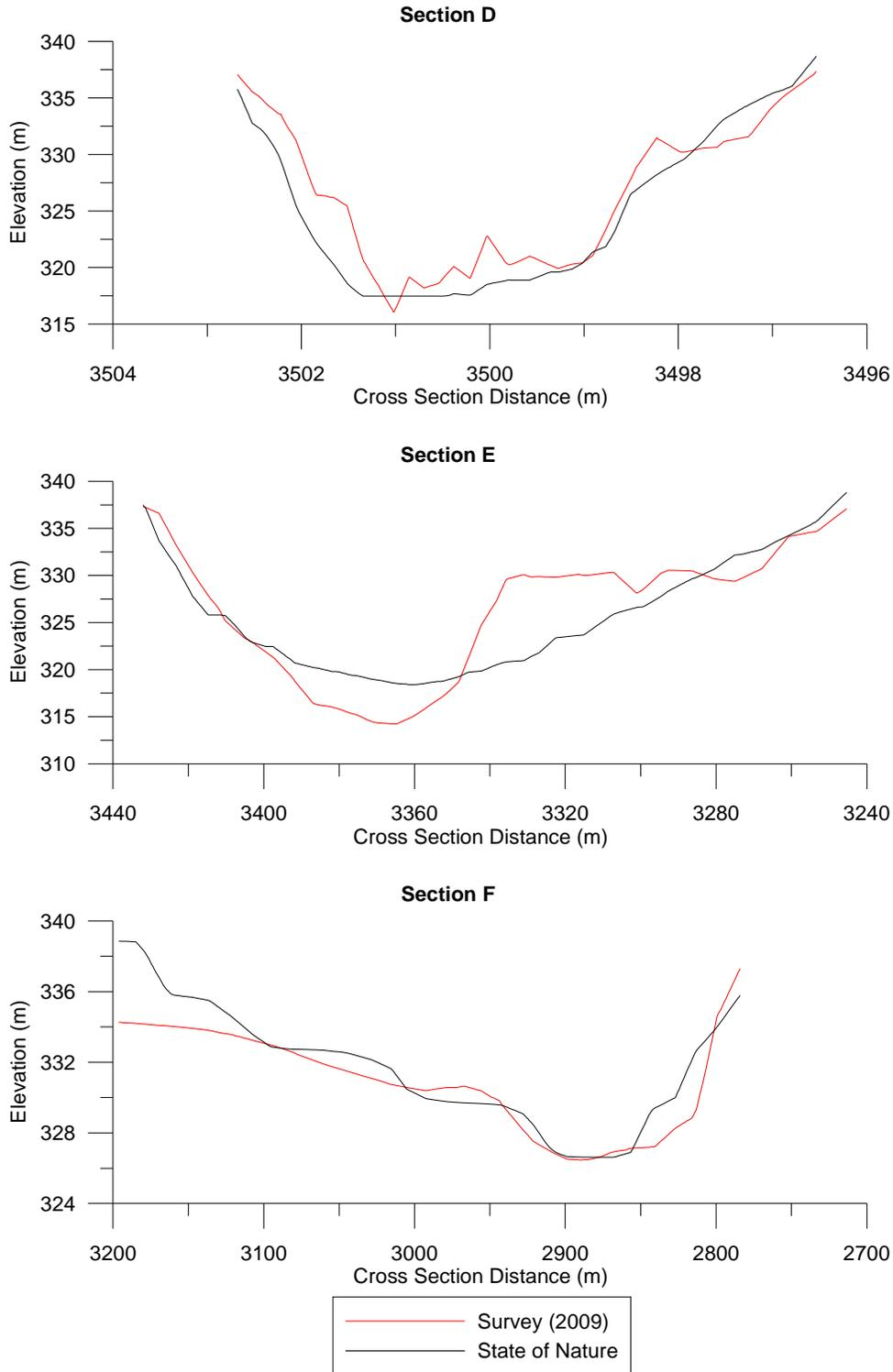
Figure D-3 - State of Nature Cross Section Comparison - D,E,F
