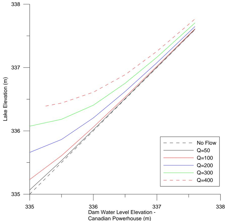
**Figure 5-4 - Rainy River HPG, Cases 1.1 and Case 2.1,  $Q < 400 \text{ m}^3/\text{s}$**
