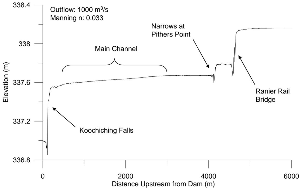
Figure 4-1 - Water Surface Elevation Profile - Regions of Hydraulic Loss
