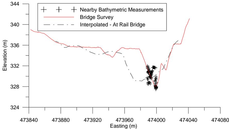
**Figure A-4 - Bridge survey cross section with nearby bathymetric measurements**
