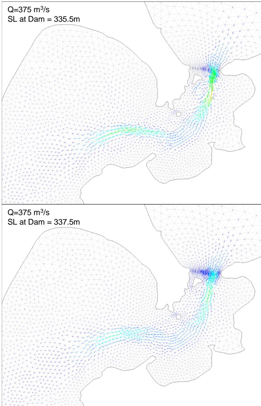
Figure 5-2 - Ranier Rapids Flow Profiles, Q = 375 m<sup>3</sup>/s
