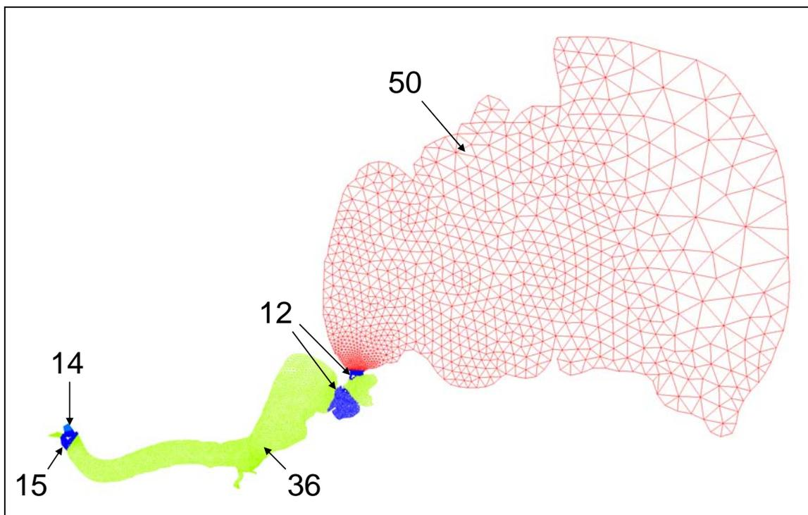
**Figure 4-3 - Calibrated Roughness Map – Mesh 1 (Strickler Coefficient)**
