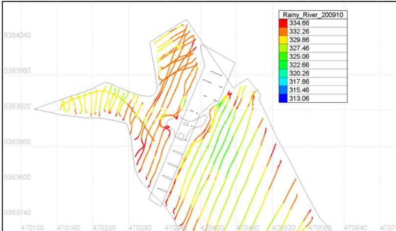
**Figure 2-5 - EC Bathymetric Survey - International Falls Bridge**
