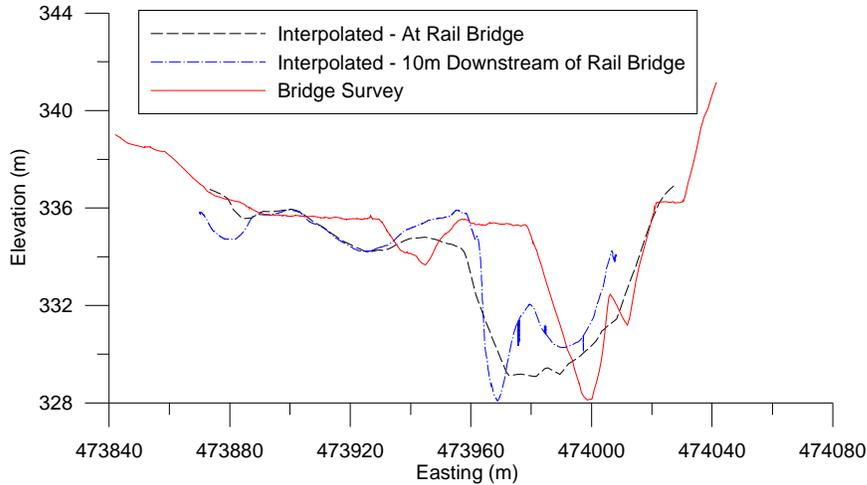
**Figure A-3 - Bathymetric Cross Sections near Rail Bridge**
