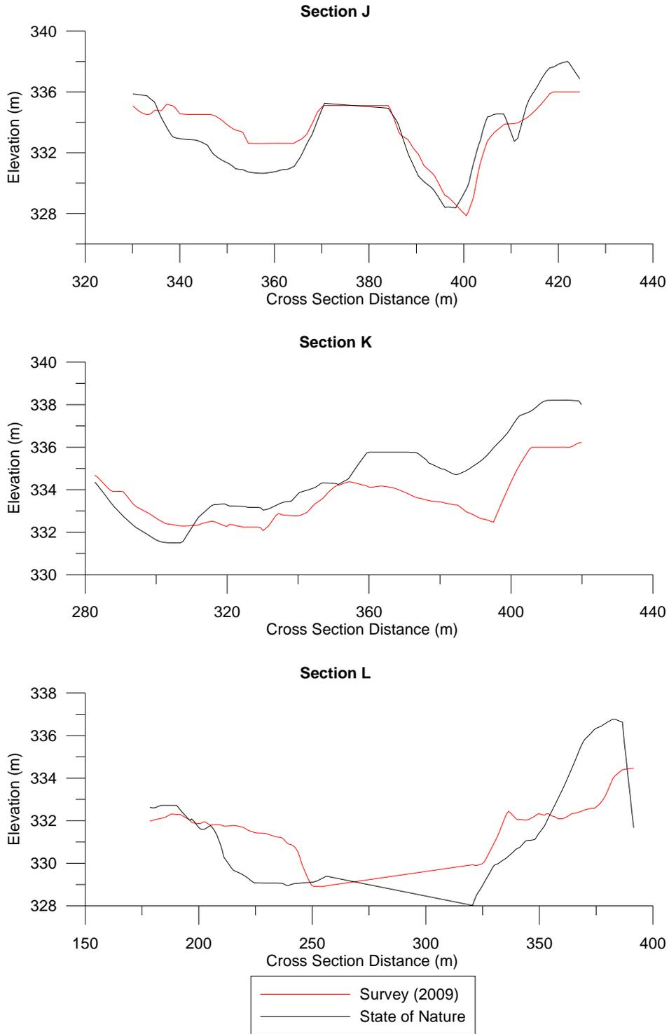
Figure D-5 - State of Nature Cross Section Comparison - J,K,L
