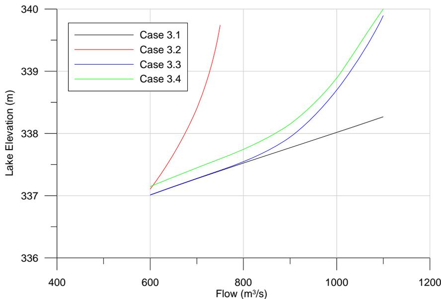
**Figure 5-5 - Steady-State Flow-Lake Level Relationships**
