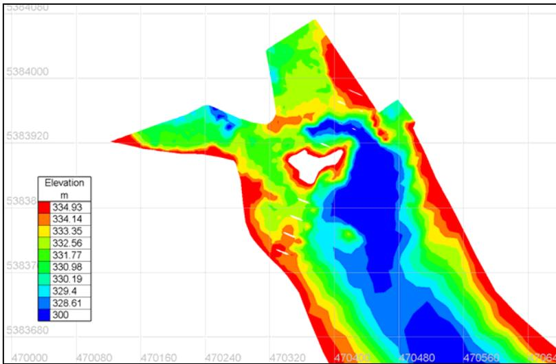
**Figure 2-10 - Interpolated Bathymetry at International Falls Bridge**
