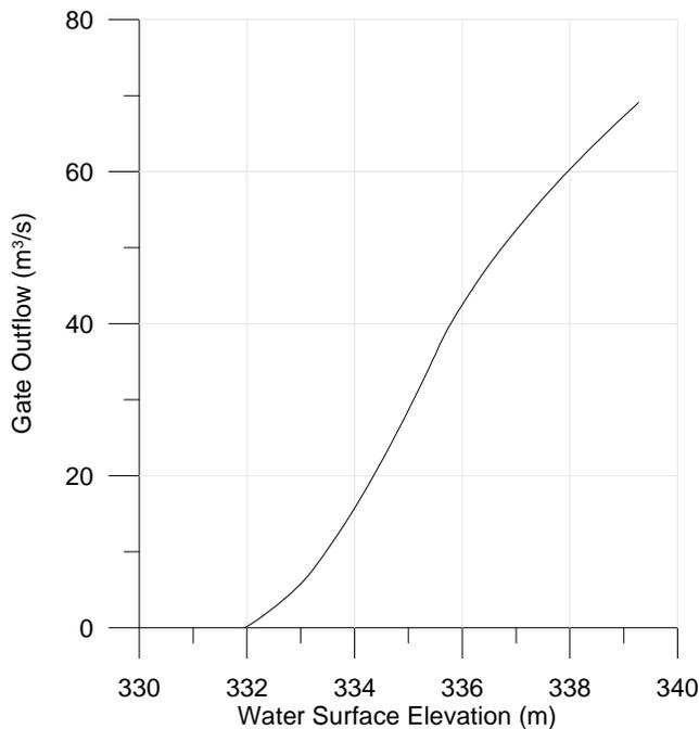
**Figure 3-5 – Individual Gate Outflow Rating Curve**
