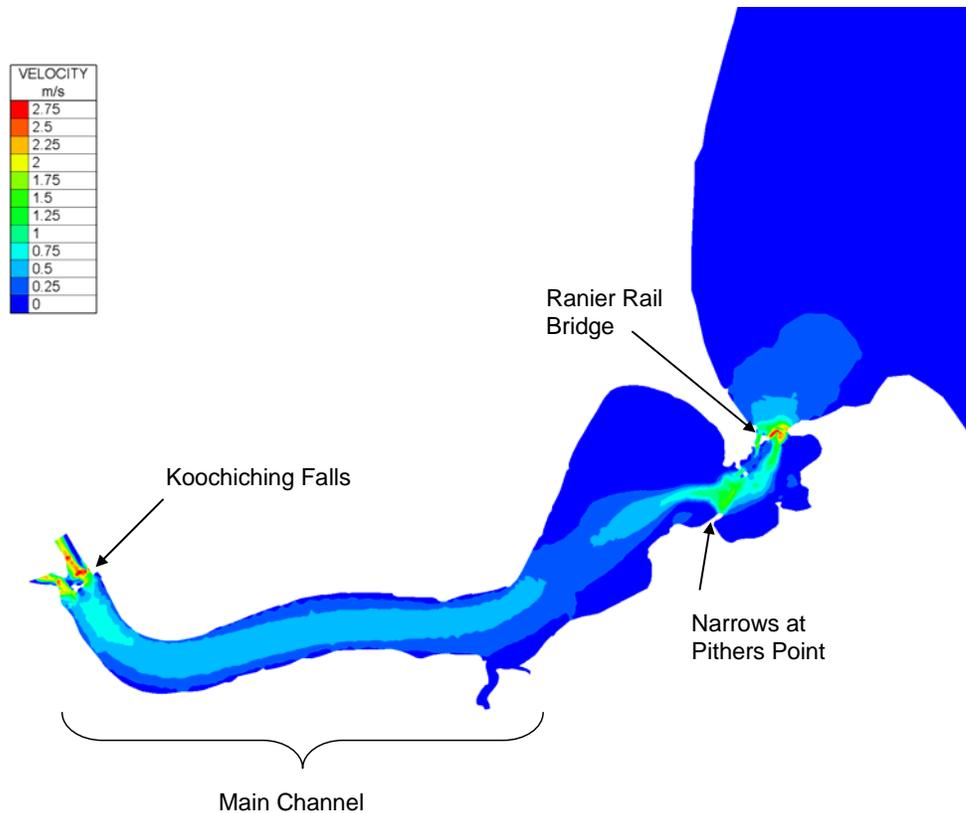
**Figure 4-2 - Velocity Map – Locations of Hydraulic Loss (Outflow = 1000 m<sup>3</sup>/s)**
