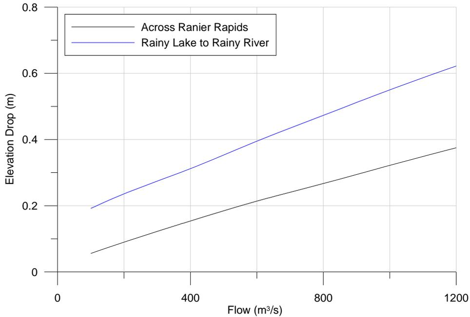
**Figure 5-14 - State of Nature - Elevation Drop by Flow Rate**
