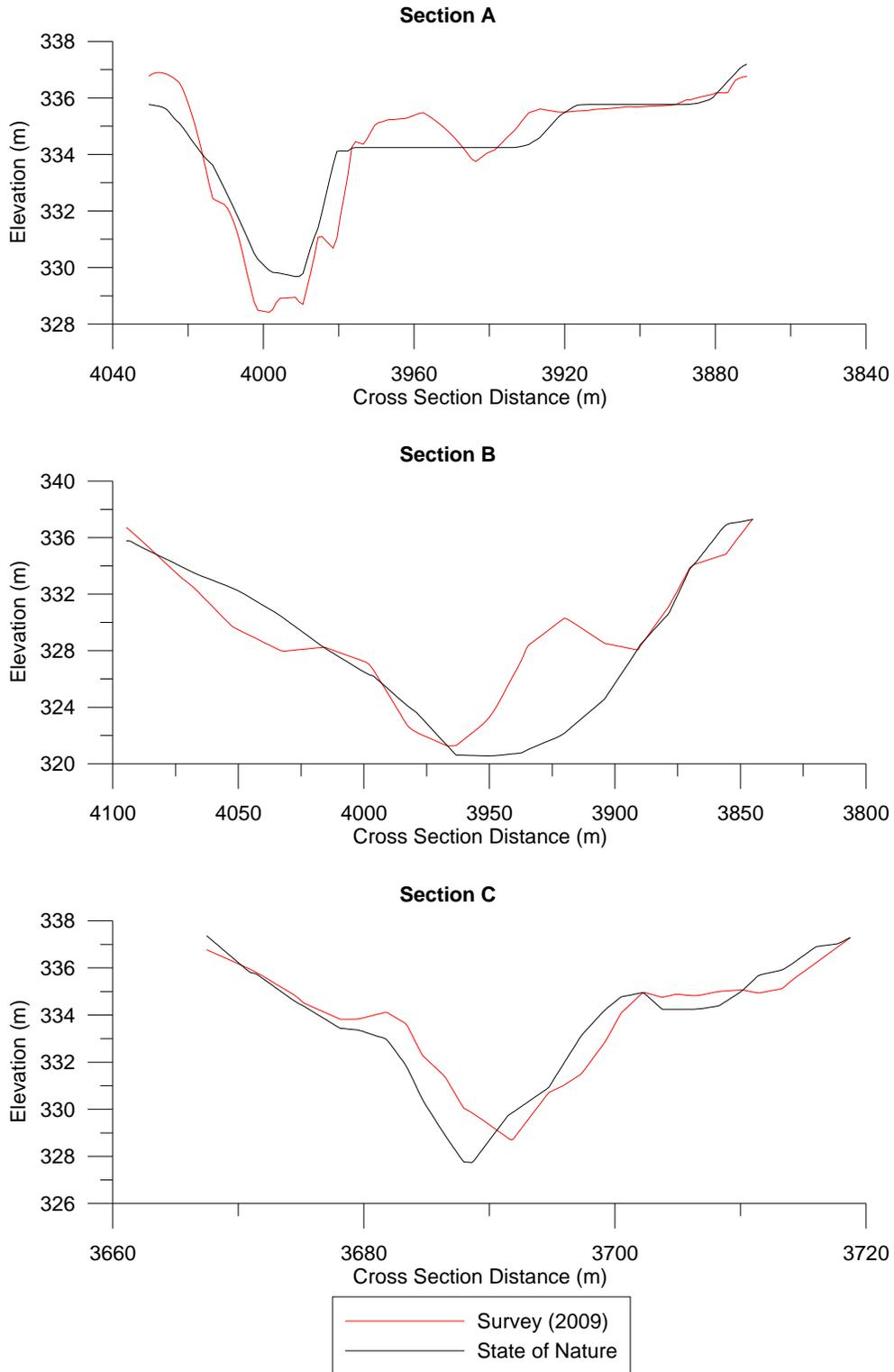
**Figure D-2 - State of Nature Cross Section Comparison - A,B,C**
