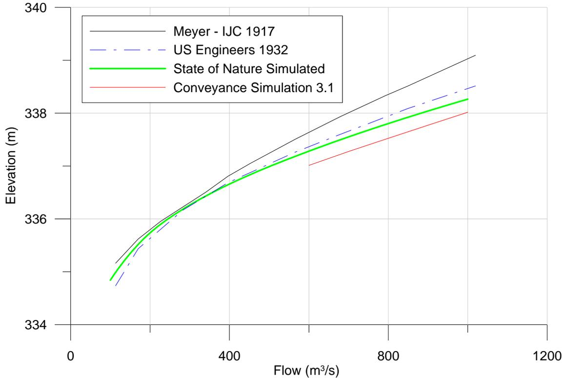
**Figure 5-15 - Rating Curve Comparison for Rainy Lake Levels in a State of Nature**
