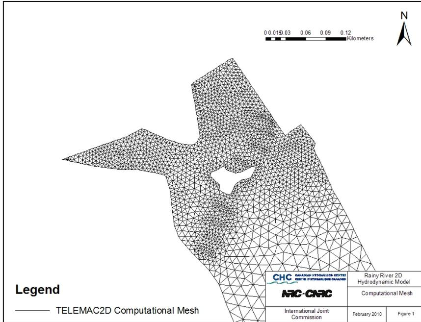
**Figure B-2 - 2D Computational Mesh - International Falls Bridge (Mesh 1 and Mesh 2)**
