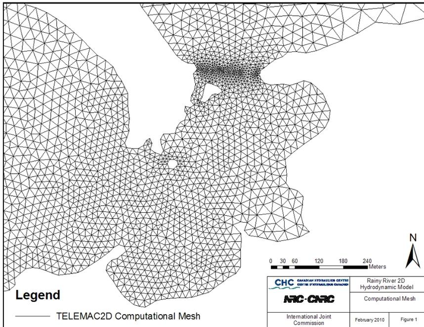
**Figure B-3 - 2D Computational Mesh - Rainier Rapids (Mesh 1 and Mesh 2)**
