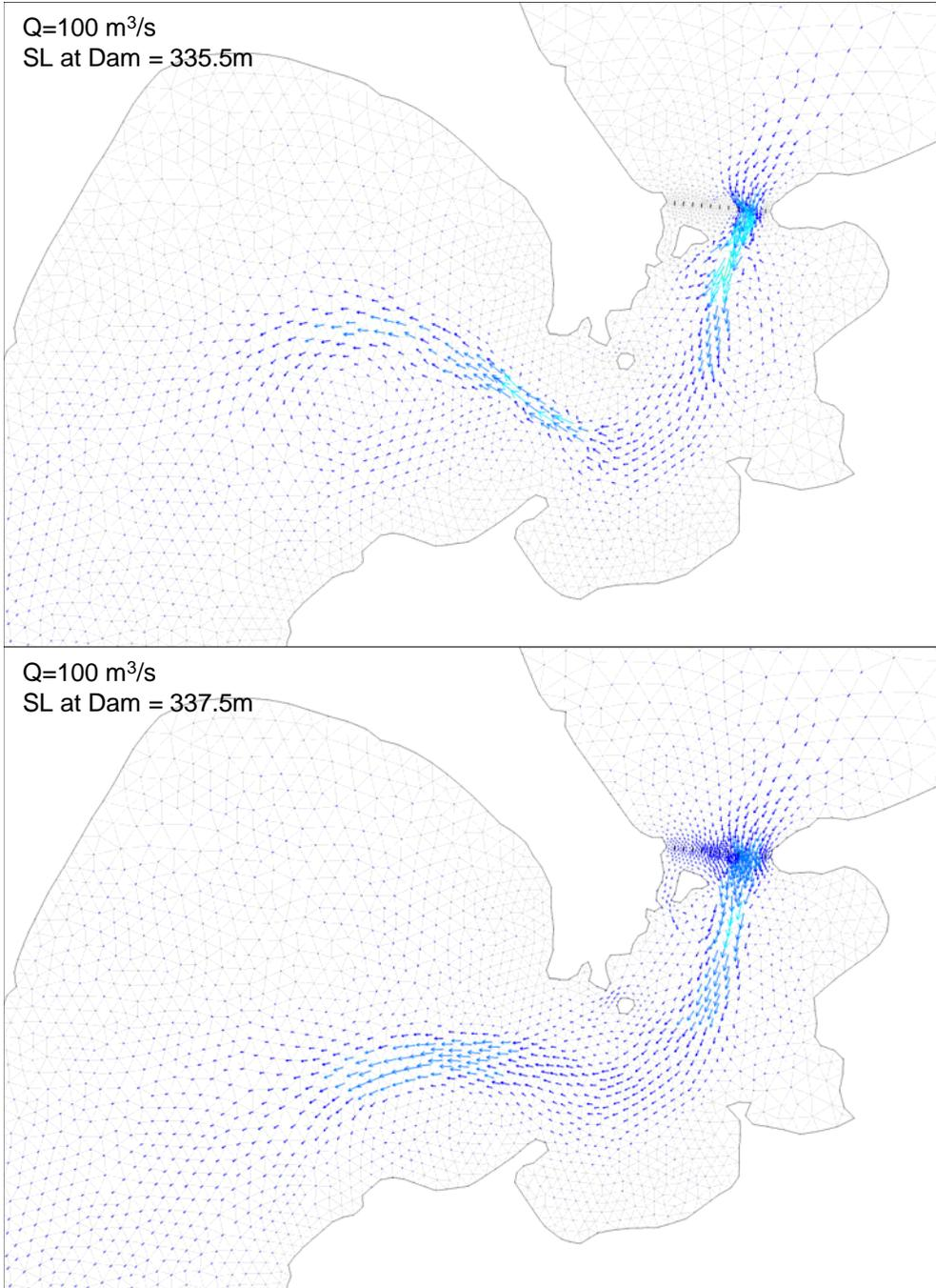
**Figure 5-1 - Ranier Rapids Flow Profiles, Q = 100 m<sup>3</sup>/s**
