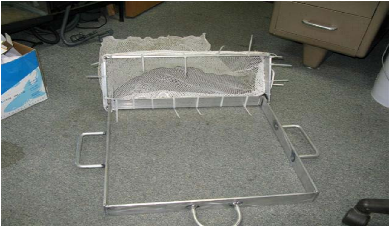
Figure 4. 1/4\text{m}^2 sampler used to collect all substrate at each sample site.
