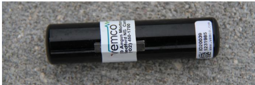
Figure 3: Vemco V16-4H acoustic transmitter used in telemetry study.
