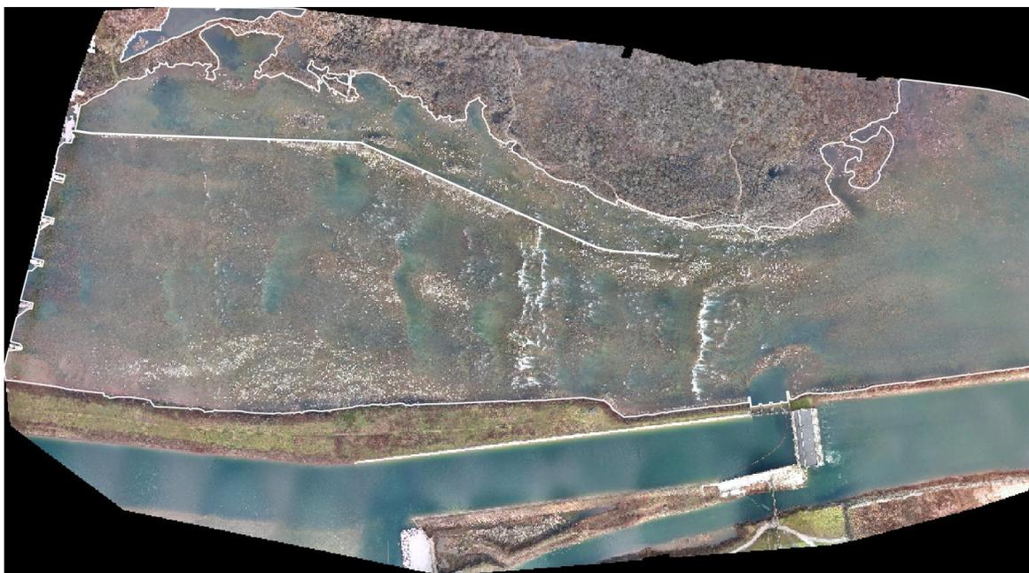
Figure 8: Compound image obtained from multiple aerial pictures shot from an Unmanned Aerial Vehicle flying over a trans-border stretch of the St-Mary's River located north of Edison Sault Hydroelectric Plant (Michigan, USA; +45.5062,-84.3493). Dimensions (x × y): 1197 m × 659 m, resolution: 4.455 cm . White lines represent the limit of the water mask used for the analysis.
